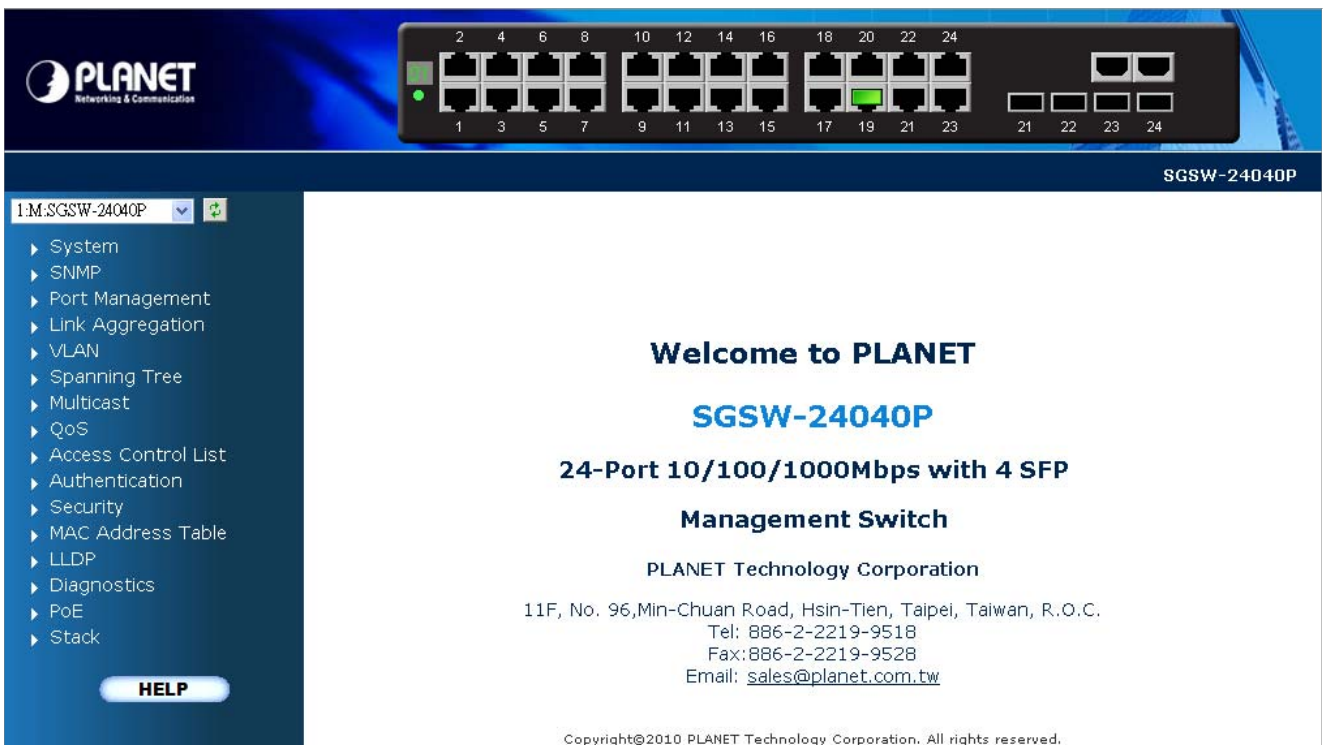
Figure 3-4 Web main screen of Managed Switch
